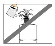
DO NOT allow water to splash or run on to the back of the fridge/ freezer. Water impairs the insulation of the electrical parts and may cause an electric short circuit or risk of electric shock.
